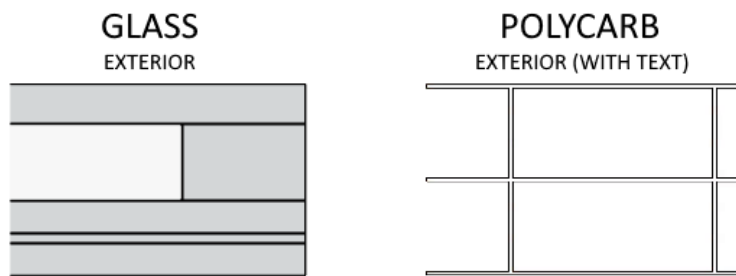
Edge View of Glazing- note which side goes to exterior.
