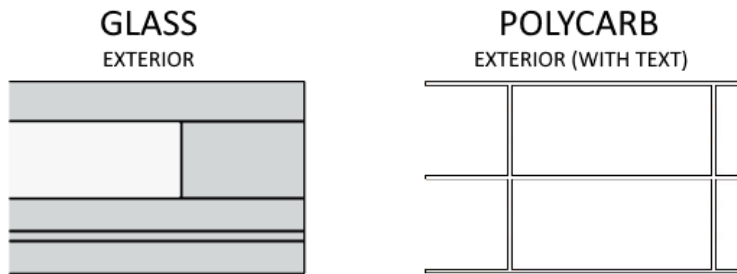
Glazing- note which side goes to exterior.
